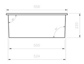
NB: Due to manufacturing processes this sink may have a +/- 4mm tolerance on the measurements.
